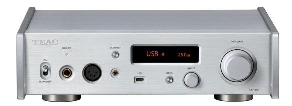
The UD-507 also incorporates TEAC's QVCS (Quad Volume Control System), a high-precision analog volume attenuator. This system, along with a powerful high-current line buffer circuit, ensures precise volume control and robust signal integrity. The dual monaural configuration of the analog output stage, with independent D/A converter sections for the left and right channels, enhances channel separation and stereo imaging.
